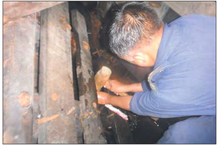
ICG repairing hull of FB Rekha Sagar
