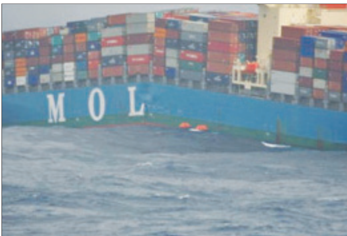
MV Mol Comfort breaking into two parts
