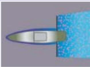
Bow wave as well as ship pitch push the oil away from the vessel and out of reach of the spray booms. Furthermore, the bow wave must not herd the dispersant before it has had a chance of penetrating the oil. The more viscous the oil is, the longer it takes the dispersant
