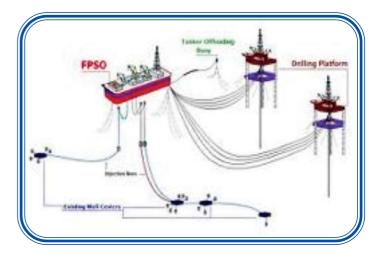
attached to the seafloor, instead of up on the platform. The extracted petroleum is transported via risers from this wellhead to the production facilities on the semisubmersible platform. These production systems can operate in water depths of up to 6,000 feet.
