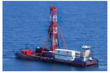
swamps, rivers, and canals. Drilling barges are large, floating platforms, which must be towed by tugboat from location to location. Suitable for still, shallow waters, drilling barges are not able to withstand the water movement experienced in large open water situations.
