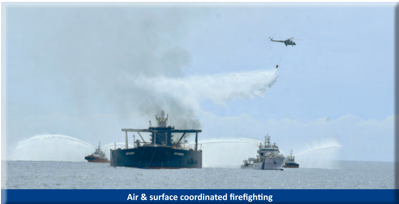
Firefighting & boundary cooling
